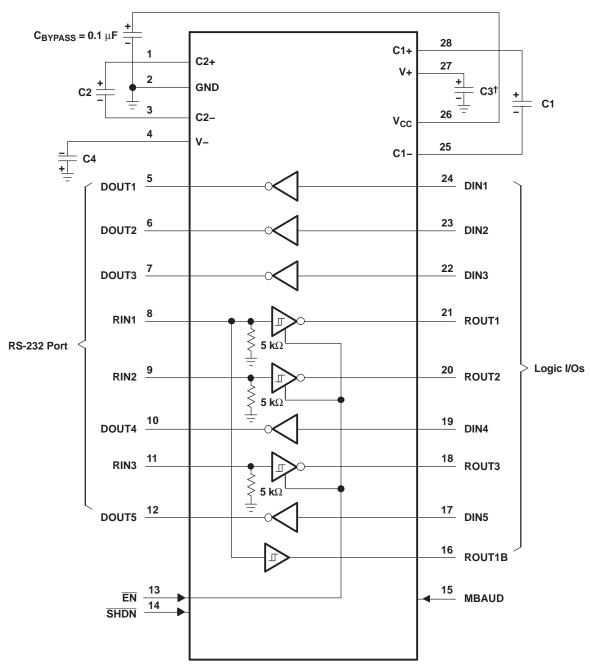
$<sup>^{\</sup>dagger}$  C3 can be connected to  $V_{CC}$  or GND.
