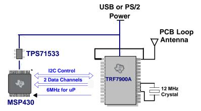
The TRF7900A simplifies system design by reducing system component count and manual circuit tuning. By integrating the PLL, SAW filter, and RF mixer, the TRF7900A eliminates the manual tuning of RLC circuits required in traditional implementations.
