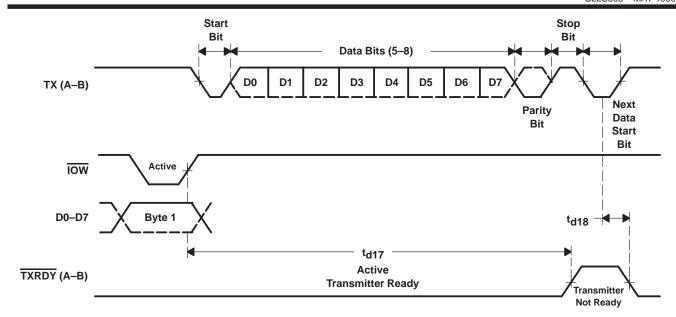
Figure 18. Transmit Ready Timing in None FIFO Mode
