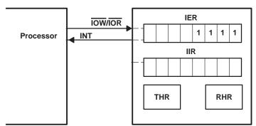
Figure 5. FIFO Interrupt Mode Operation
