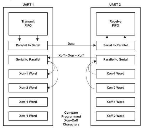
Figure 4. Software Flow Control Example
