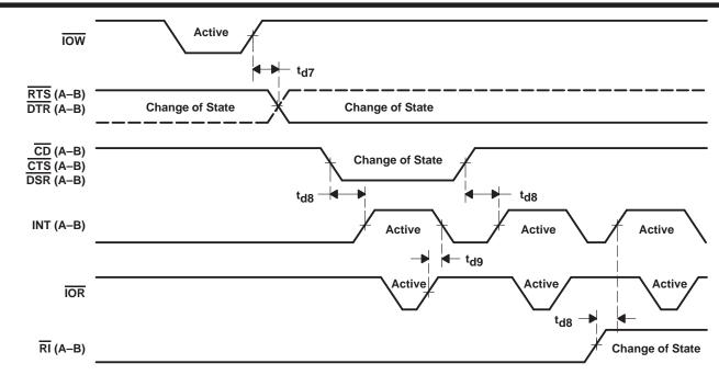
Figure 14. Modem Input/Output Timing
