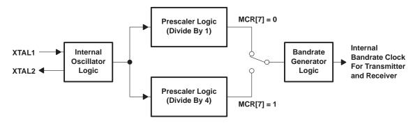
Figure 9. Prescaler and Baud Rate Generator Block Diagram
