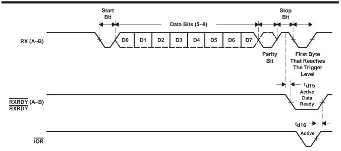
Figure 16. Receive Timing in FIFO Mode
