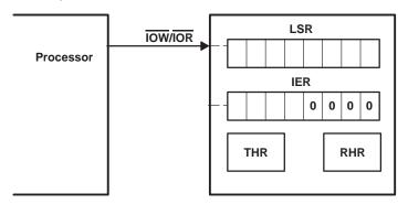
Figure 6. FIFO Polled Mode Operation
