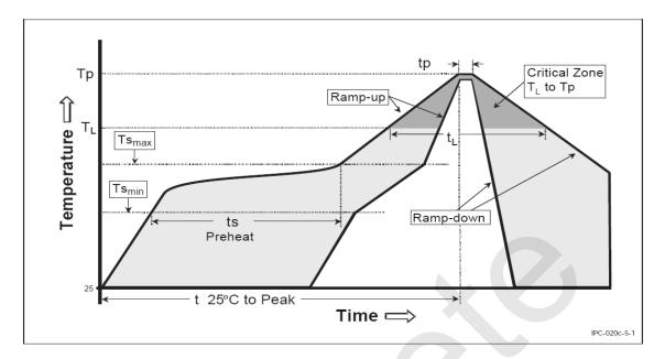
Figure 29. Typical Reflow Profiles
