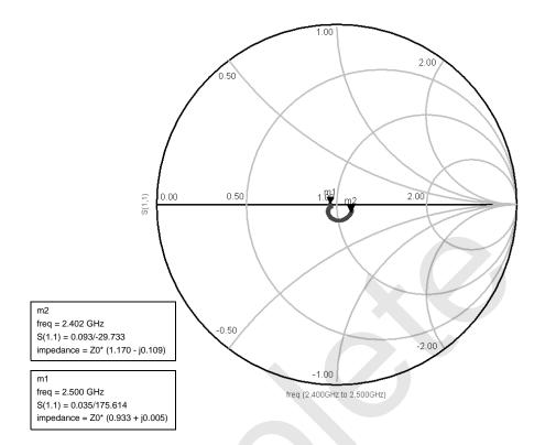
Figure 7. TX and RX Pin 50 $\Omega$  Impedance Characteristics
