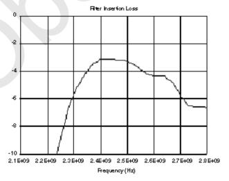
Figure 6. Front-End Bandpass Filter Response
