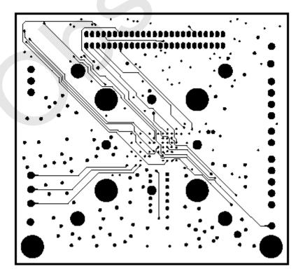
Figure 27. Signal Plane (Layer 3)
