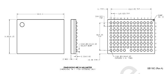
Figure 31. Package with NOPB Solder Bumps (plastic housing).
