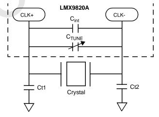
Figure 9. LMX9820A Crystal Recommended Circuit
