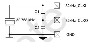
Figure 13. 32.768 kHz Oscillator
