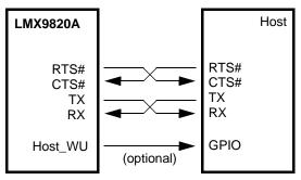
Figure 19. UART Null Modem Connections
