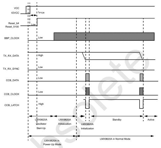
Figure 16. LMX9820A System Power-Up Sequence Timing
