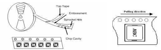
Remark: The sprocket holes are to the right as the tape is pulled toward the user.
