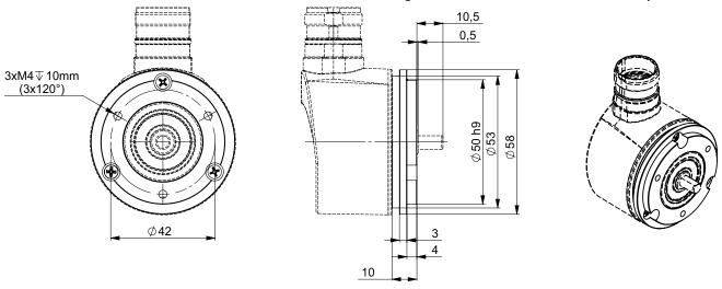
DHM5\_10 Connection G3R (Radial cable), flange 9500/005 mounted on the body
