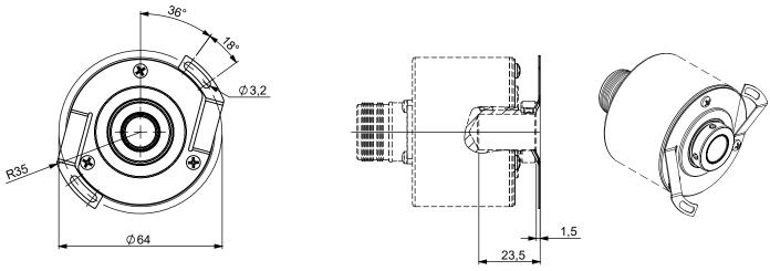
DHO5\_14 Standard clamping, Connection G3R (Radial Cable), coupling 9445/012 mounted on the body
