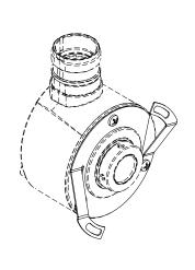
DHO514 Flange side clamping, Connection U3R (Radial cable), coupling 9445/068 mounted on the body
