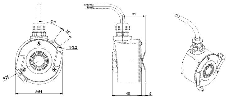
DH05\_14 Standard clamping, Connection G3R (Radial Cable), coupling 9445/015 mounted on the body
