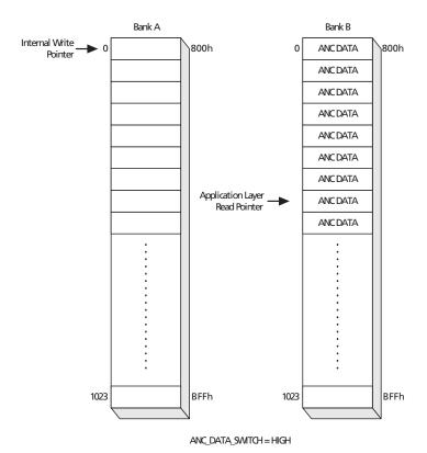
Figure 4-24: Ancillary Data Extraction - Step D
