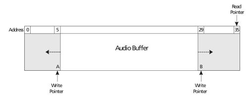
Figure 4-36: Audio Buffer Pointer Boundary Checking
