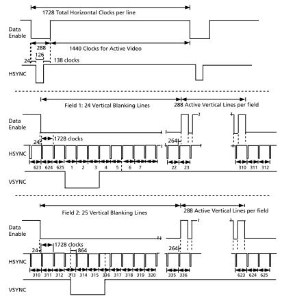
Figure 4-16: H:V:DE Output Timing 720 (1440) x 576 @ 50 (Format 21 & 22)
