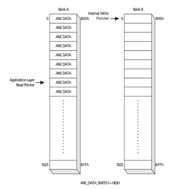
Figure 4-22: Ancillary Data Extraction - Step B
