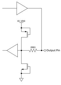
Figure 3-3: Bidirectional Digital Input/Output Pin with programmable drive strength. These pins are configured to output unless in Reset Mode; in which case they are high-impedance. The drive strength can be set by writing to address 06Dh in the host interface register. (DOUT0, DOUT1, DOUT2, DOUT3, DOUT4, DOUT5, DOUT6, DOUT7, DOUT8, DOUT9, SDOUT\_TDO, STAT0, STAT1, STAT2, STAT3, STAT4, STAT5, XTAL\_OUT, DOUT10, DOUT11, DOUT12, DOUT13, DOUT14, DOUT15, DOUT16, DOUT17, DOUT18, DOUT19, PCLK)
