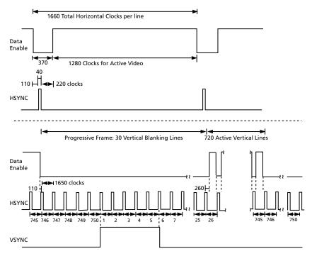
Figure 4-11: H:V:DE Output Timing 1280 x 720p @ 59.94/60 (Format 4)
