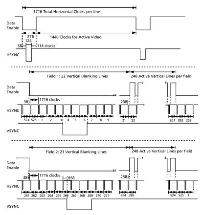
Figure 4-13: H:V:DE Output Timing 720 (1440) x 480i @ 59.94/60 (Format 6&7)
