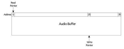
Figure 4-35: Audio Buffer After Initial 26 Sample Write
