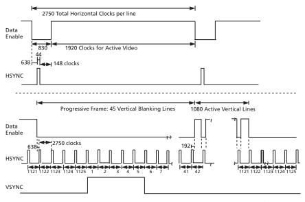
Figure 4-17: H:V:DE Output Timing 1920 x 1080p @ 23.94/24 (Format 32)
