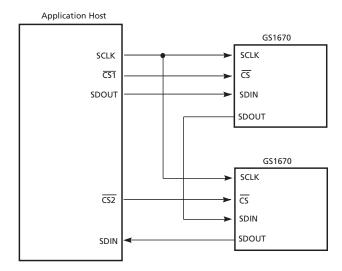
Figure 4-37: GSPI Application Interface Connection
