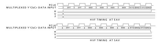
Figure 4-8: H:V:F Output Timing - HD 10-bit Output Mode
