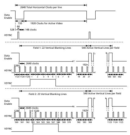
Figure 4-15: H:V:DE Output Timing 1920 x 1080i @ 50 (Format 20)
