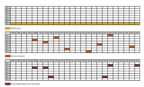
Figure 4-33: ECC 24-bit Array and Examples
