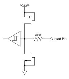
Figure 3-1: Digital Input Pin with Schmitt Trigger (20bit/10bit, AUDIO\_EN/DIS, CS\_TMS, SW\_EN, IOPROC\_EN/DIS, JTAG/HOST, RC\_BYP, RESET\_TRST, SCLK\_TCK, SDIN\_TDI, SDO\_EN/DIS, STANDBY, TIM\_861)
