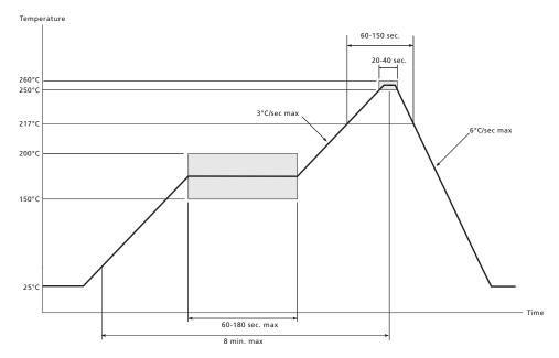
Figure 7-1: Pb-free Solder Reflow Profile
