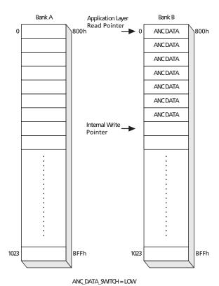
Figure 4-23: Ancillary Data Extraction - Step C
