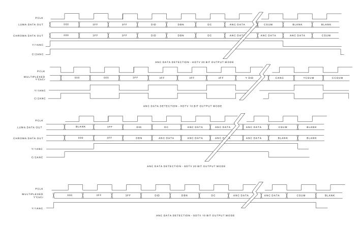
Figure 4-20: Y/1ANC and C/2ANC Signal Timing
