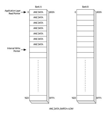
Figure 4-21: Ancillary Data Extraction - Step A
