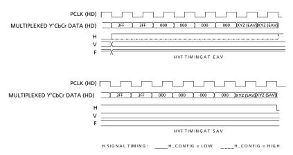
Figure 4-6: H:V:F Output Timing - HDTV 10-bit Mode
