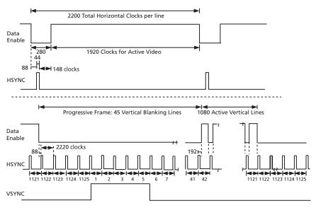
Figure 4-19: H:V:DE Output Timing 1920 x 1080p @ 29.97/30 (Format 34)
