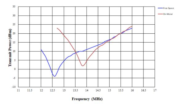
\*HF sensitivity shown in the figure is measured by Voyantic Tagformance HF Loop Antenna C60 on 15\*15mm steel plate. Actual sensitivity performance is subject to the environment in practice.
