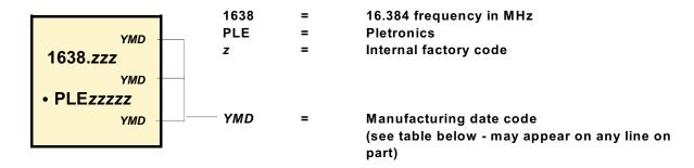
The actual part number is THD3004-16.384M where the model number "004" is the specification number the part is made to. This is not included in the part marking. This is included on the label on the Tape and Reel.
