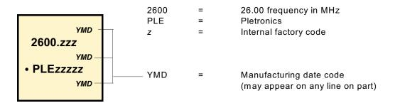
The actual part number is TCD4027-26.0M where the model number "027" is the specification number the part is made to. This is not included in the part marking. This is included on the label on the Tape and Reel.
