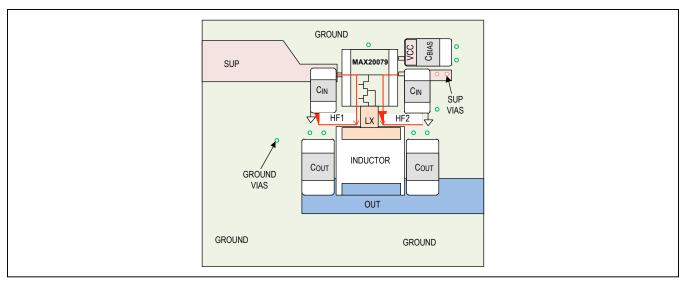
Figure 2. Recommended PCB Layout for MAX20079
