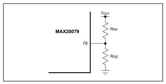
Figure 1. Adjustable Output-Voltage Setting
