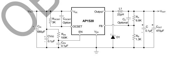
Note:  $V_{OUT}=V_{FB} \times (1+R_A/R_B)$  $R_B=0.7k\Omega$  to  $5k\Omega$
