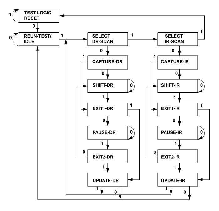
Figure 1. TAP Controller State Diagram<sup>[21]</sup>
