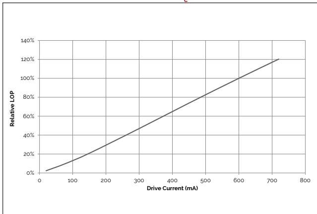
Figure 3: Vesta Dim-to-Warm 13mm 20W Relative LOP vs. Drive Current, T_c = 25^\circ\text{C}
