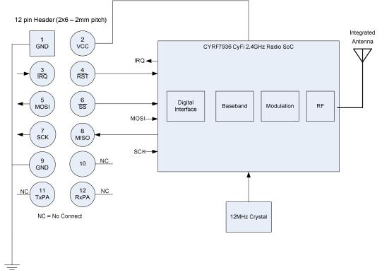
\*Figure 1 – Module Schematic (Header version)
